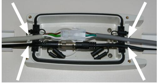
12. Use the plugs attached to seal the cable attachment points that are now not required (see illustration on the right).
