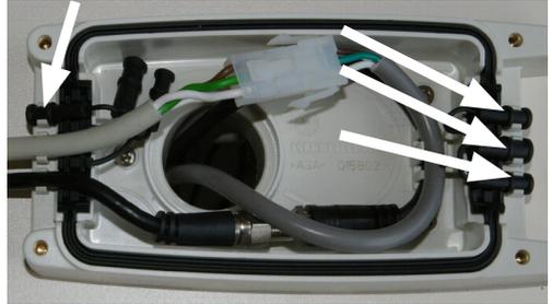
12. Now place the cover on the casing lower half and screw the two halves together using the four screws pre-inserted in the cover (tightening torque:  $M_A = 1-1.5 \text{ Nm}$ ).
